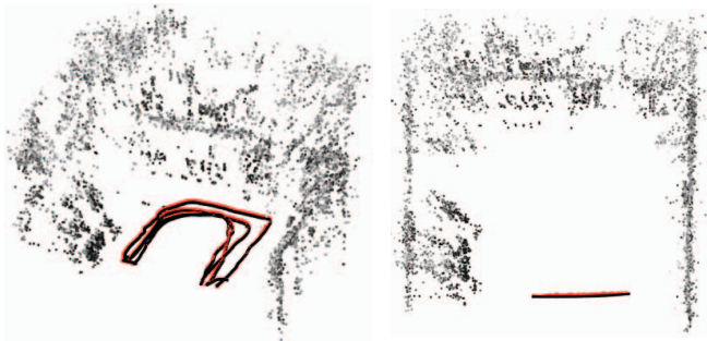
Fig. 10. 'Circle' (left) and 'Sideways' (right) trajectories estimated by our method (in red) are very similar to the ground truth trajectories (in black).
