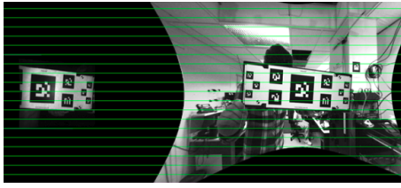
Figure 9. : Depth camera image rectified into visual camera frame of reference. Green lines show matching points on each image.
